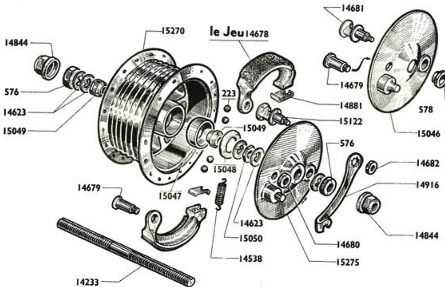
ROUE AVANT ET MOYEU AVANT "PRIOR"
