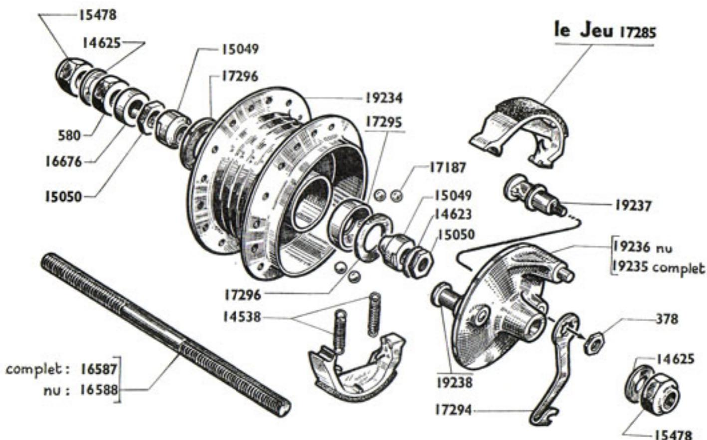
ROUE ET MOYEU AVANT "PRIOR" Ø 80  $\frac{m}{m}$
