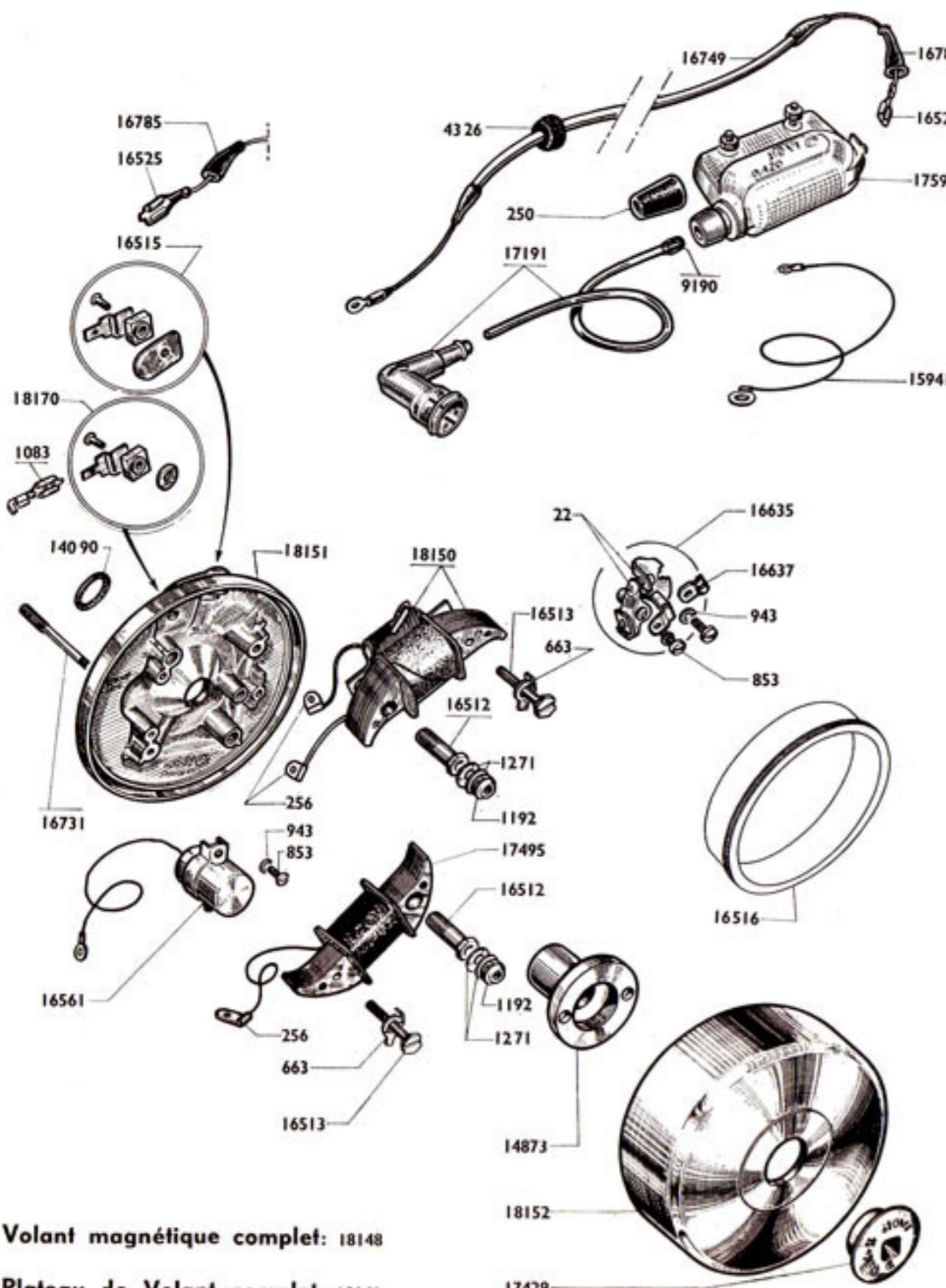
VOLANT MAGNETIQUE (25 + 3 watts)
